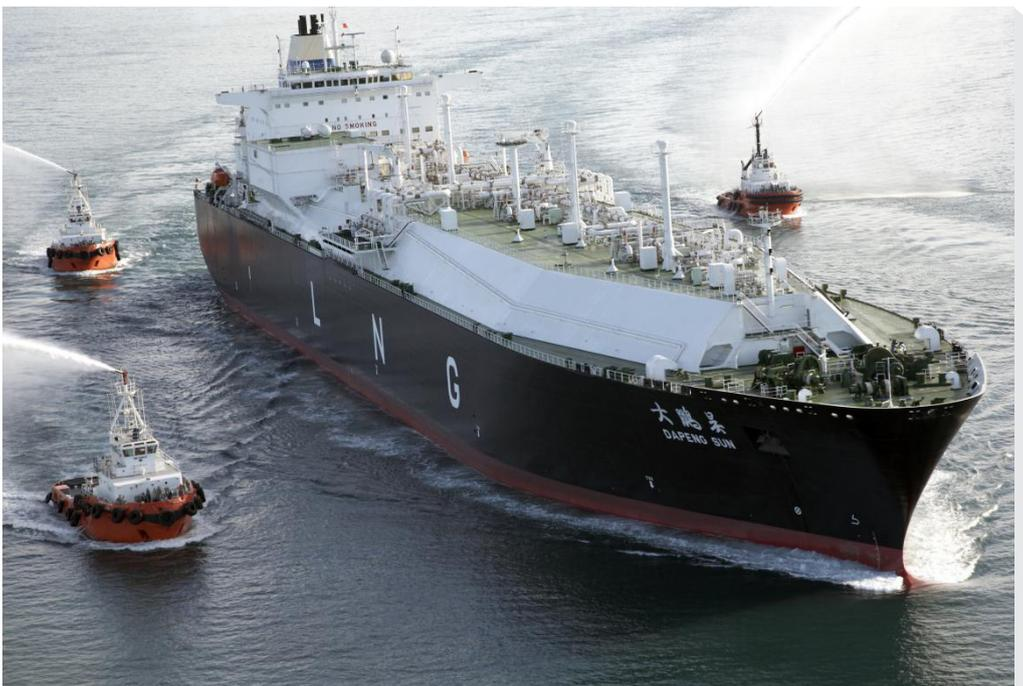
A membrane-type LNG carrier with a capacity of 147,000 cu m built by China
