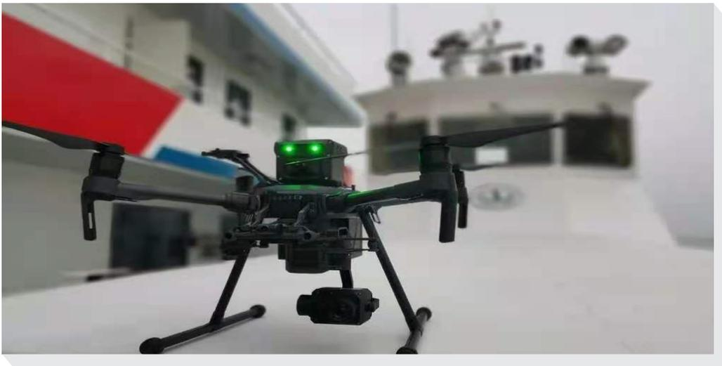
Ship exhausts remote sensing drone and airborne sniffing equipment
