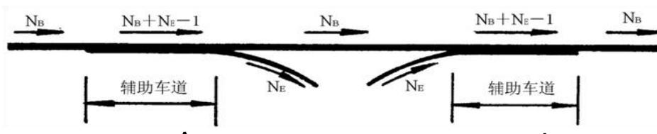
Fig. 11.4.3 Auxiliary Lanes at two-lane Exit/Entrance
