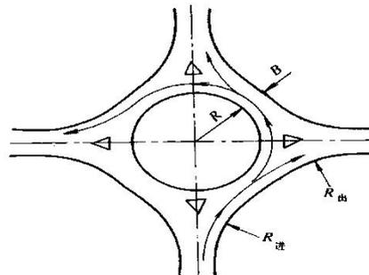
Fig. 10.1.4 Channelization (placing traffic islands)
