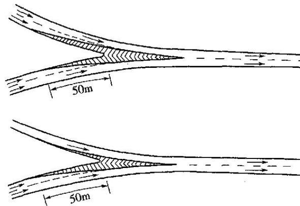
**Fig 11.5.4 Lane Reduction before Merging**
