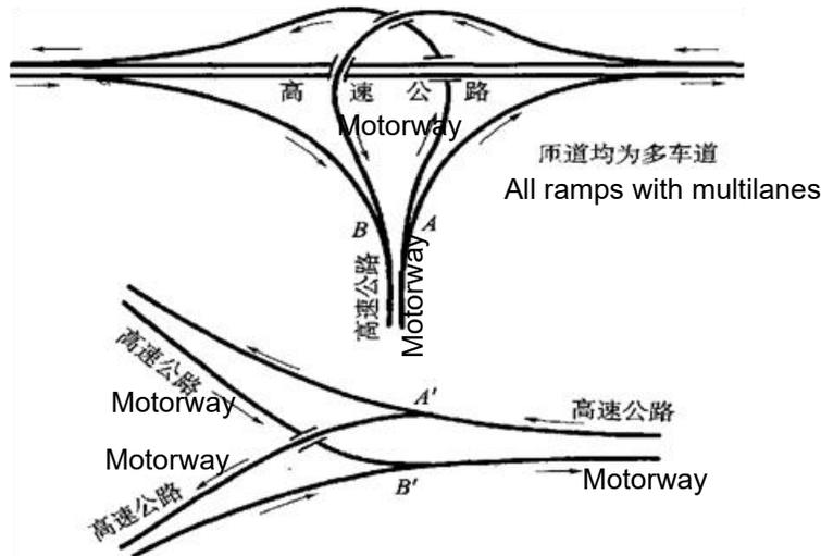
**Fig. 11.5.1 Diverging and Merging of Main Route**
