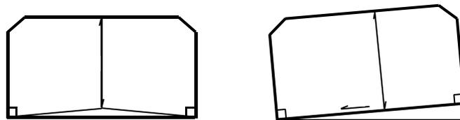
a) a normal crowned section    b) a superelevated section
