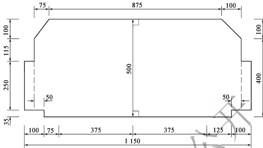
Fig. B.0.9-1 Clearance of expressway two-lane tunnel (120km/h) (dimensions given in cm)
