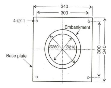
Figure 1.2.2.3-2 - Cylindrical vessel, 200 mm diameter
