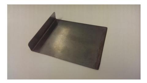
Figure 1.5.5.1.9 – Typical scraping device
