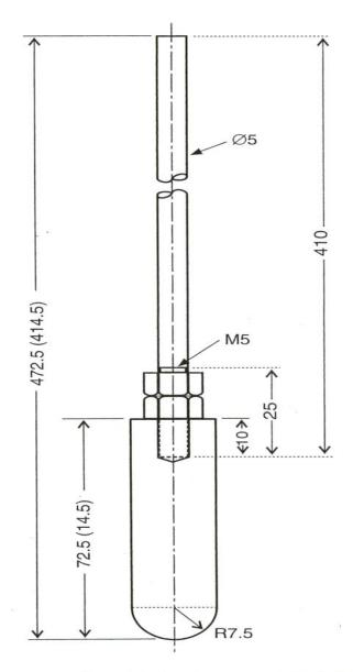
(Dimensions indicated in brackets are of the 5 kPa bit) (unit: mm)
