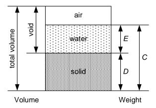
Figure 1.5.5.3.1 – Illustration of key variables
