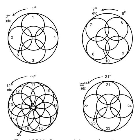
Figure 1.5.5.3.2 – Recommended compaction patterns
