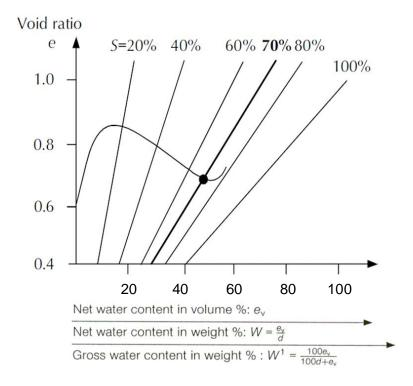
Figure 1.5.5.3.6 – Typical compaction curve
