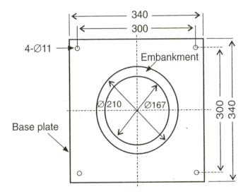
Figure 1.2.2.3-1 - Cylindrical vessel, 150 mm diameter
