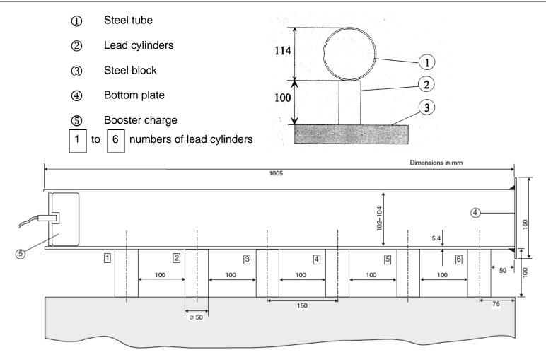
Figure 2 – Positioning of the steel tube on the firing site
