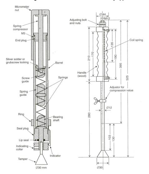
Figure 1.1.2.4 – Examples of spring-loaded tampers
