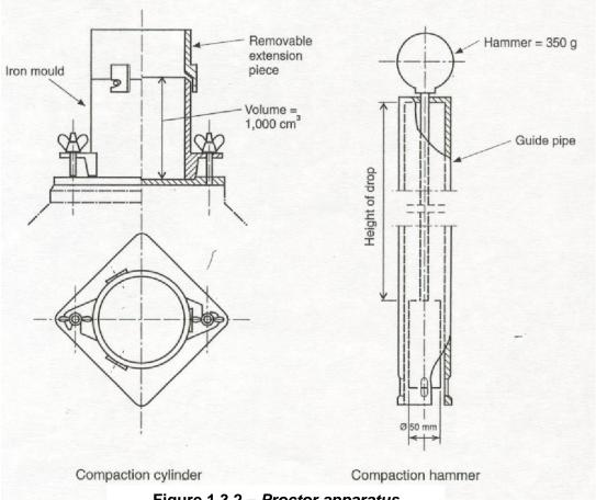
Figure 1.3.2 – Proctor apparatus
