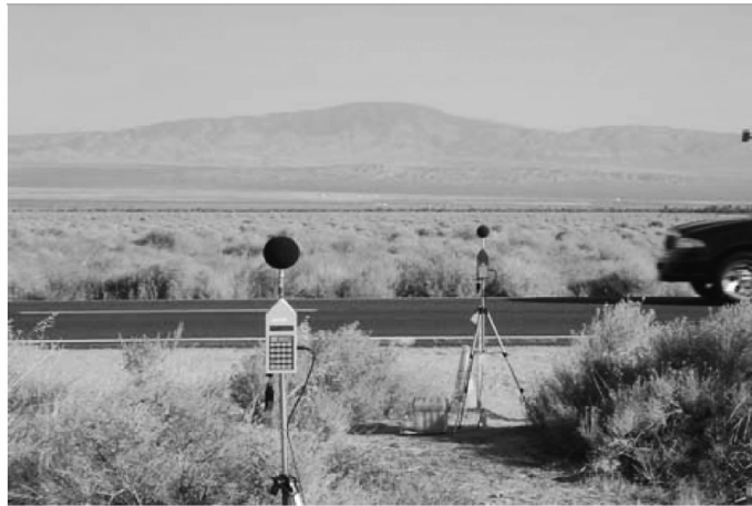
Figure T 0986-5 Set up of traffic noise test under far-field method
